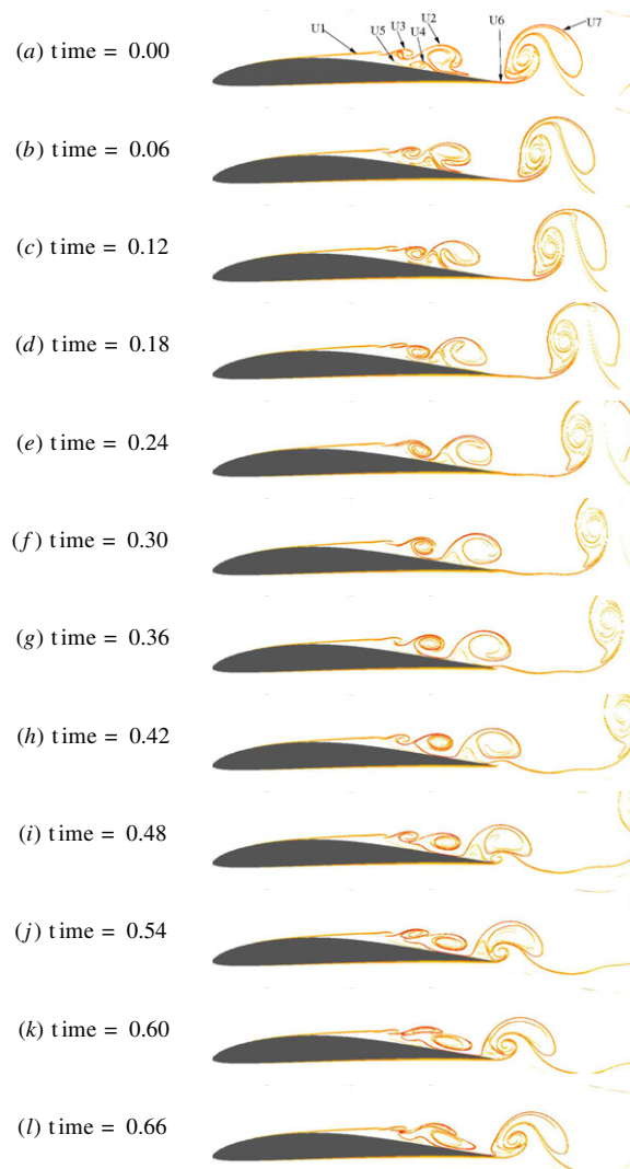
Figure 4. Contour plots of FTLE over airfoil, U1–U7 are the major recurring structures in the flow, online version shows these ridges in red and orange.
