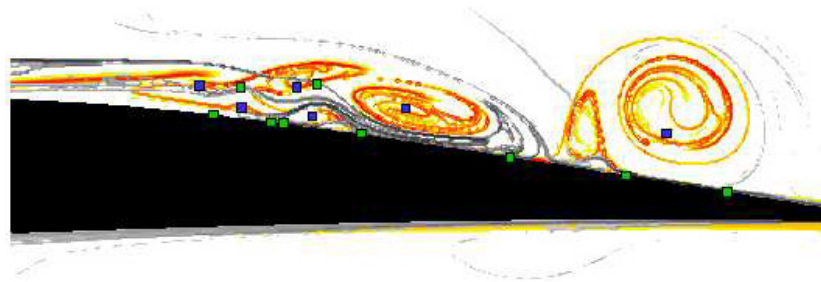
Figure 18. Fixed points in the flow, overlaid on top of stable and unstable manifolds. Online version shows unstable manifolds in red, stable manifolds are overlaid in gray. Hyperbolic fixed points are gray squares (green online) ( \blacksquare ), elliptic fixed points are black squares (dark blue online) ( \blacksquare ).
